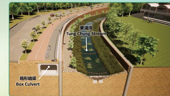
東涌河和箱形暗渠的橫切面模擬圖 Photomontage of the cross section of Tung Chung Stream and box culvert
